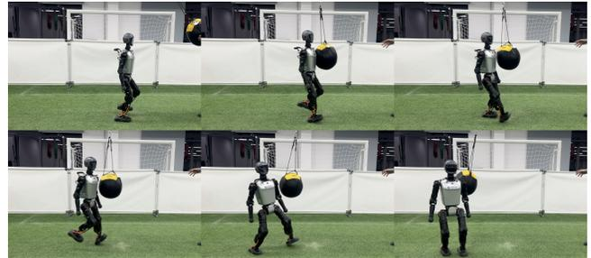
Fig. 6: Push Recovery. A 10-kg ball impacts the robot during stepping in place. The robot regains a stable gait within a few steps after the disturbance.
